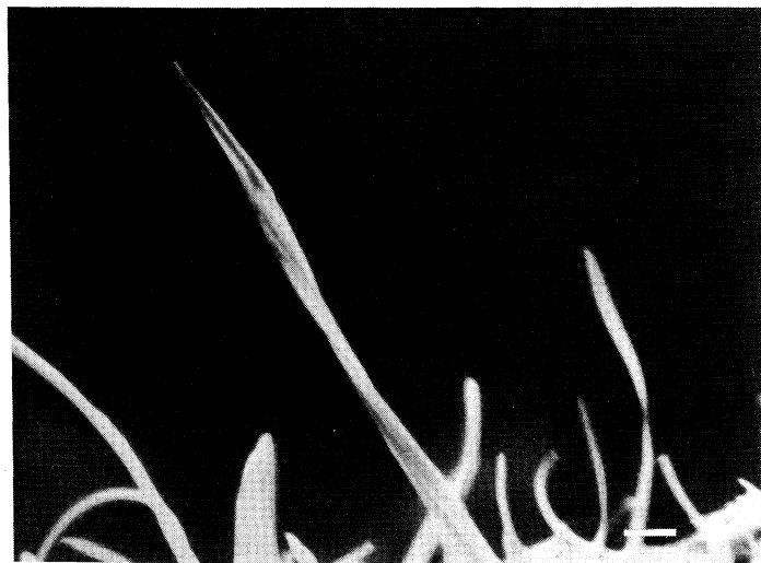
Fig. 6. Electron micrograph of anneal gel of D-DBS/ethylene glycol (scale bar 1 \mu\text{m} ).
